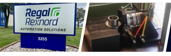
Spin testing under load ensures against defects to each bearing's rollers or raceway.
