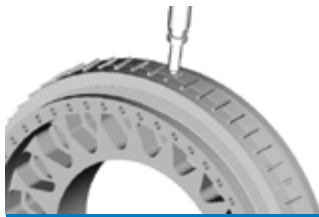
Powerlign/Powerwheel pick up teeth shown with one sensor (second not shown is at 180°.)
