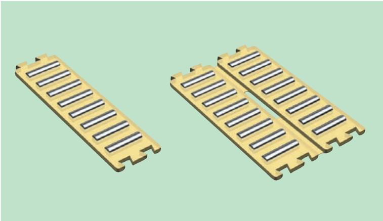
This flat roller bearing, comprised of a flat cage and needle rollers, reciprocates on a flat raceway by motion of linear movable components.
