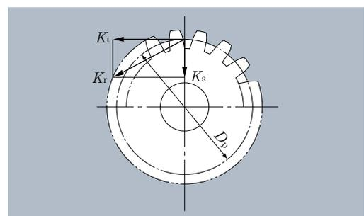
**Fig. 3.3** Composite radial force acting on gear
