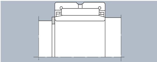
**Fig. 8.6** Inner ring fixing method with snap ring
