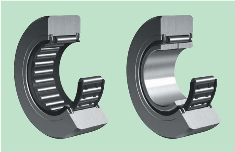
This roller follower is a bearing designed for rotation of the outer ring. A needle roller and cage assembly and a synthetic rubber seal reinforced with steel plate are assembled in a thick-walled outer ring.
