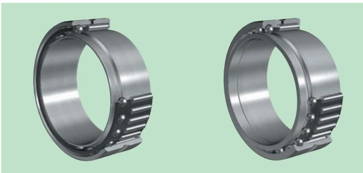
This complex bearing is comprised of a needle roller bearing for supporting radial load, a ball bearing for supporting comparatively small axial load and machined inner and outer rings which are all assembled integrally. Both angular contact ball bearing and three-point contact ball bearing are available to support the axial load.
