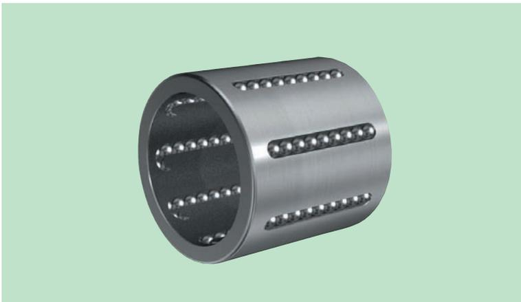
The product assembly includes an outer ring formed through precision deep-drawing of thin sheet steel material, steel balls, and a synthetic resin cage that retains the steel balls. This high-precision linear motion bearing develops infinite linear motion on the shaft.
