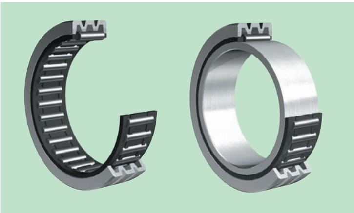
This product is essentially comprised of a machined outer ring, inner ring, and, needle rollers with a cage to guide the rollers. This product features an outer ring with a unique cross-sections shape machined from a solid blank material. With this bearing, the roller and cage assembly cannot be separated from the outer ring. If the user wants to use the shaft directly as a raceway surface, **NTN** offers a variant that lacks inner ring.
