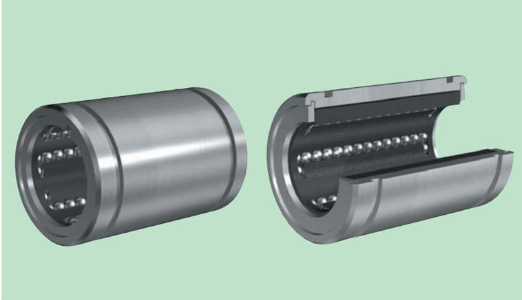
The product assembly includes a machined outer ring, side plate, steel balls, and a synthetic resin cage that retains the steel balls. This high-precision linear motion bearing develops infinite linear motion on the shaft.
