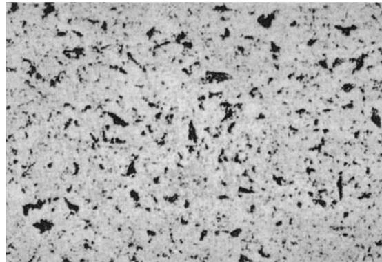
**Fig. 12.2** Magnified photo showing HL roller surface
