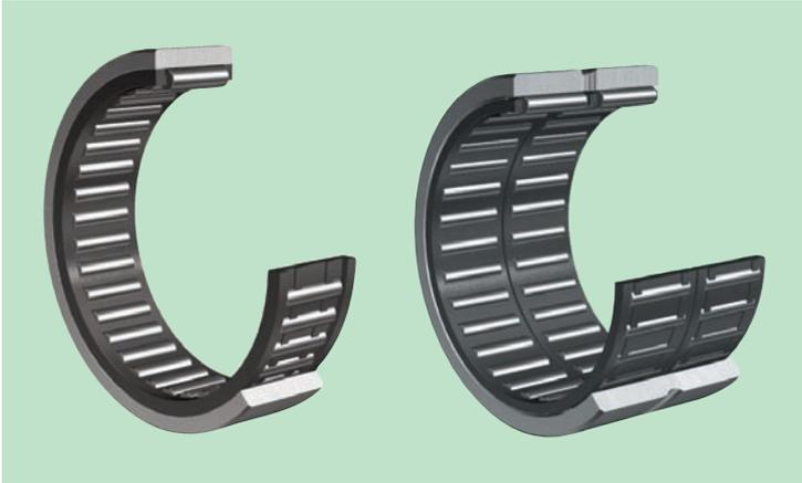
This product is essentially comprised of a machined outer ring, inner ring, and, needle rollers with a cage to guide the rollers. With this bearing, the roller and cage assembly can be separated from the outer ring. If the user wants to use the shaft directly as a raceway surface, **NTN** offers a variant that lacks inner ring.
