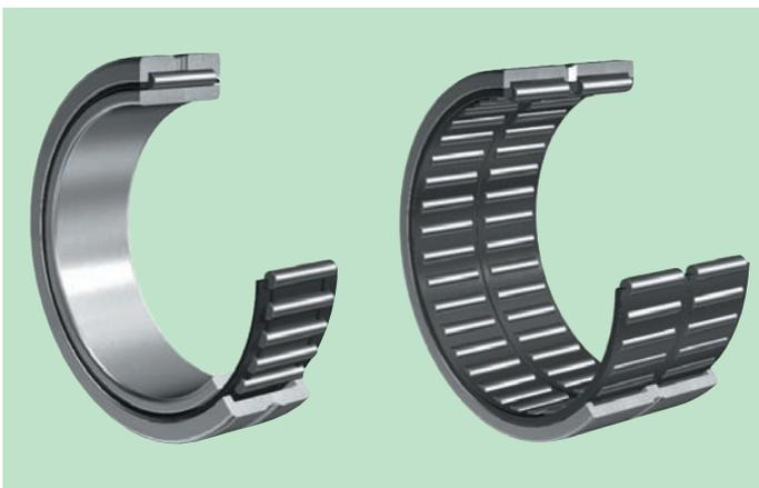
This product mainly includes machined components — an outer ring and inner ring, needle rollers and a cage that guides the rollers. In this bearing, the cage or needle rollers are guided by the rib or side plate of the outer ring. Consequently, the roller and cage assembly cannot be separated from the outer ring. When the user wants to use the shaft as the raceway surface, **NTN** can offer a variant without an inner ring.
