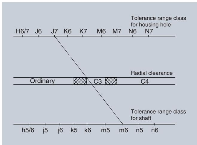
**Fig. 5.1 Relationship between bearing fits and radial clearance**
