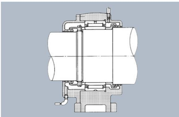
Fig.9.4 Circulating lubrication
