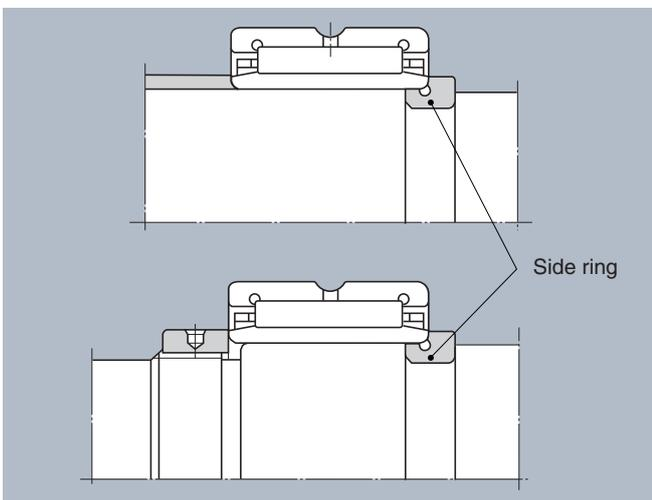
**Fig. 8.8** Inner ring fixing method with side ring
