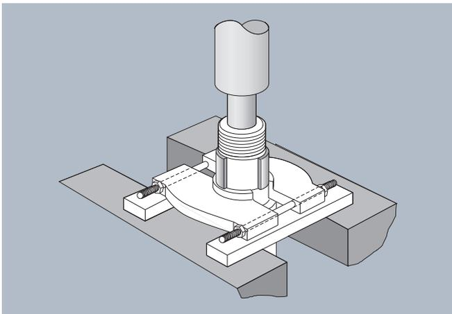
**Fig. 11.5 Bearing removal by a press machine**
