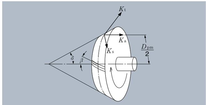
**Fig.3.5 Bevel gear diagram**
