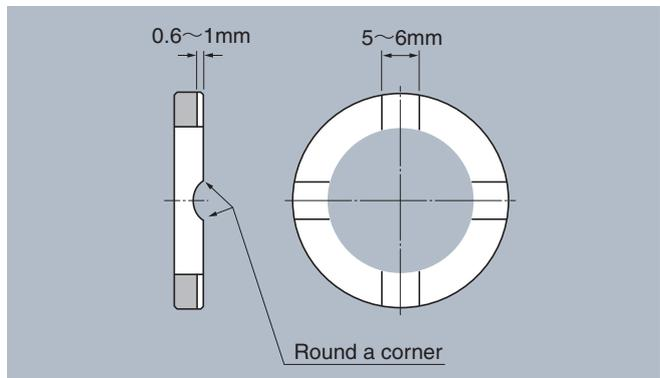
**Fig. 8.3** Design of thrust ring guide surface
