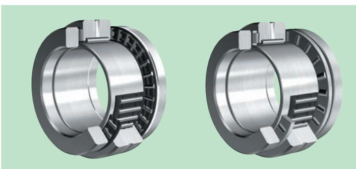
This is a complex bearing wherein a thrust needle roller bearing or a thrust cylindrical roller bearing intends to support an axial load is configured at the double sides of a radial needle roller bearing for supporting radial load.
