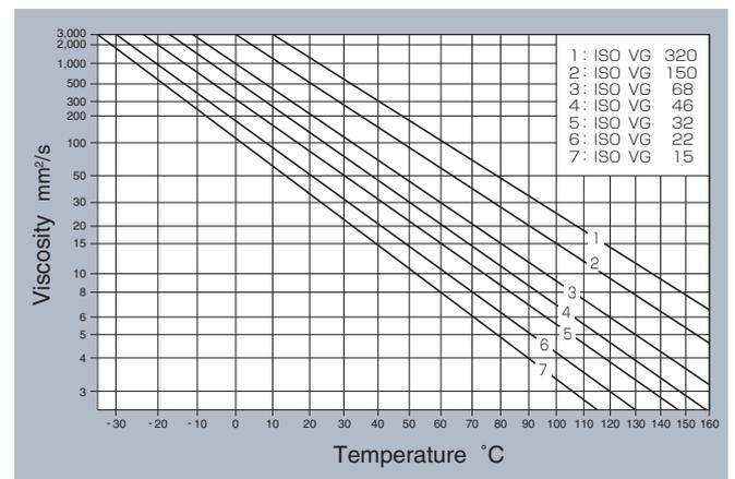
Fig. 9.5 Lubrication oil viscosity - temperature characteristic chart
