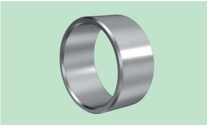
Most needle roller bearings lack an inner ring and use the shaft as raceway surface. However, there may be cases where the shaft surface cannot be changed on the machine to the required hardness and/or roughness so in this case an inner ring may be used. **NTN** inner rings are made of high carbon chromium bearing steel blank that is heat-treated, and then finish-ground to higher precision.
