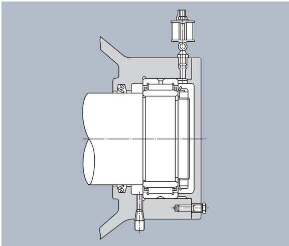
Fig. 9.3 Drip lubrication
