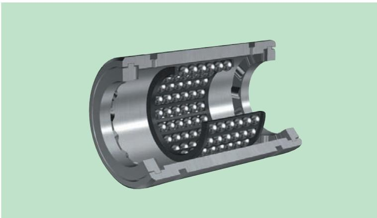
The product assembly includes a machined outer ring, side plate, steel balls, and a synthetic resin cage that retains the steel balls. This high-precision bearing rotates and develops finite linear motion on the shaft. The outer ring is provided with a snap ring on both sides and a wavy spring washer is provided between the snap ring and the cage to damp on the impact acting on the cage and to prevent wear of the cage.
