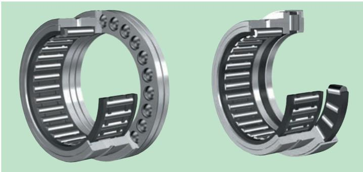
This complex bearing is comprised of a needle roller bearing for supporting radial load and a thrust bearing for supporting axial load which are assembled integrally. Both thrust ball bearing and thrust roller bearing type are available to support axial load.
