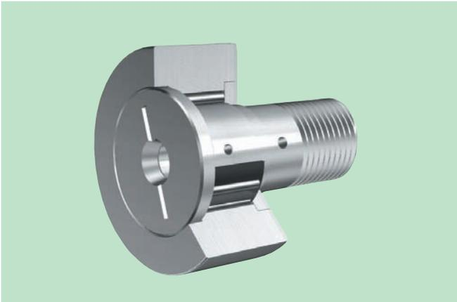
This is a bearing designed for rotation of the outer ring. A needle roller and cage assembly and a stud instead of inner ring are fitted in the thick-walled outer ring. The stud is threaded to be mounted easily. This cam follower (bearing) uses needle rollers as its rolling element and it is available with cage or full complement roller bearing type without cage.
