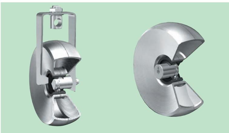
These pulleys are used to guide and tension the tapes and belts driving the spindles of a fine spinning machine, a roving frame, a false twister, etc. The structure is comprised of a precision deep-drawn plate steel pulley which is press-fitted to the outer ring of a bearing.
