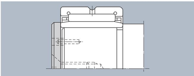
**Fig. 8.7** Inner ring fixing method with end plate
