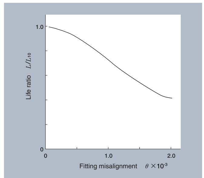
Fig. 2.8 Relationship of fitting misalignment to bearing lifetime
