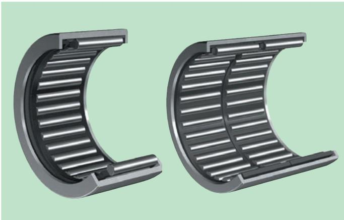
This bearing type includes an outer ring and needle rollers, which are both drawn from special thin steel plate by precision deep drawing, and a cage which guides the needle rollers precisely.
