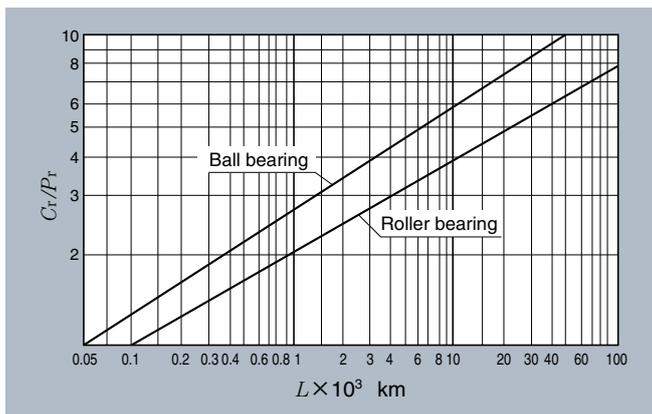
**Fig. 2.4** Life of bearing with axial motion
