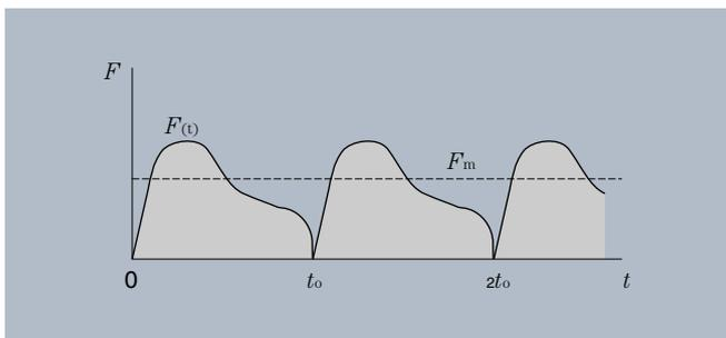
Fig. 3.9 Load fluctuating as cyclical function of time
