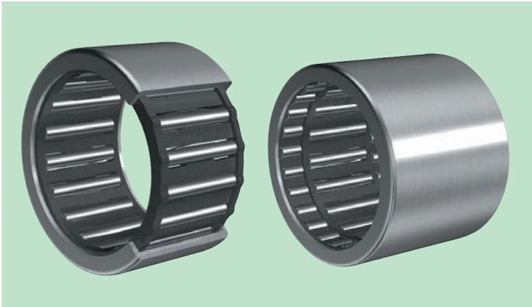
Comprised of an outer ring drawn from thin special steel plate by precision deep drawing, a spring, needle rollers and a cage, the one-way clutch can transmit torque in only one direction.
