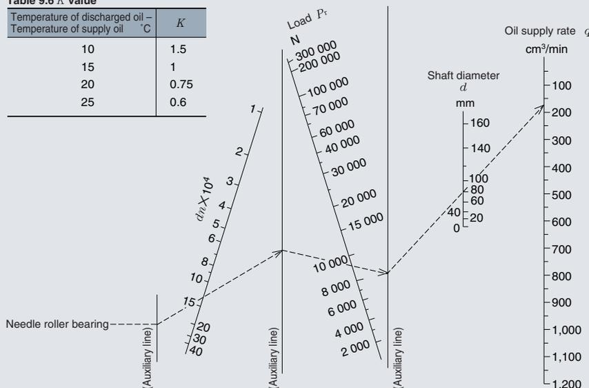
**Fig. 9.6 Chart for determining oil supply rate**
