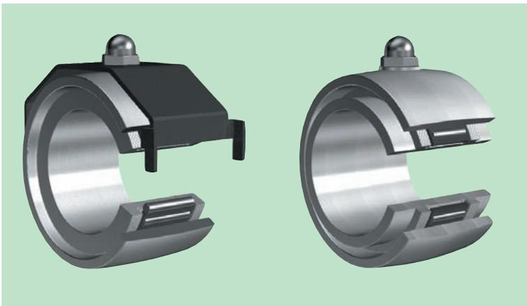
This product has a built-in needle roller bearing pre-filled with grease and is used to support bottom rollers. The spherical outer surface of the outer ring can allow a degree of bottom roller installation error. In order to prevent fiber entry into the bearing, tight clearances are maintained between the outer ring and double-ribbed inner ring, and the rib outer diameter surfaces are knurled.
