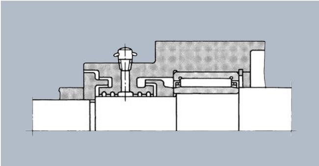
**Fig. 10.11 Combined non-contact seal**
