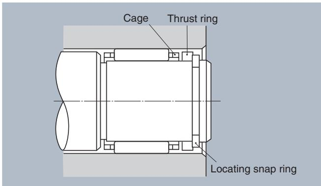
**Fig. 8.1** Bearing fixing by thrust ring
