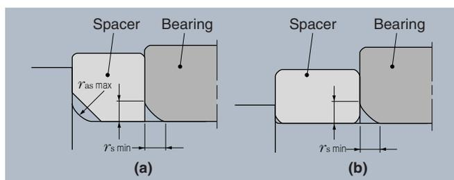
**Fig. 8.11** Spacer applications
