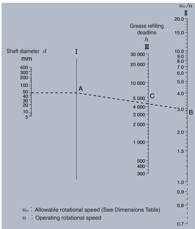
Fig.9.2 Chart for determination of grease replenishing interval
