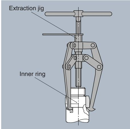
**Fig. 8.5** Inner ring extraction with extraction jig
