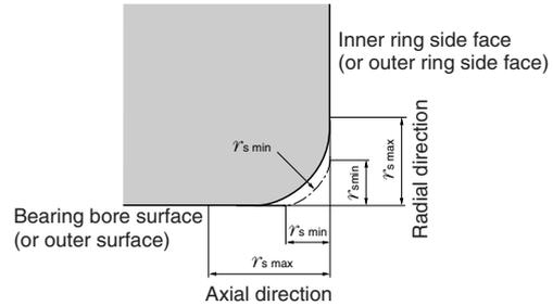
① Allowable minimum values for the chamfering dimension "r".
