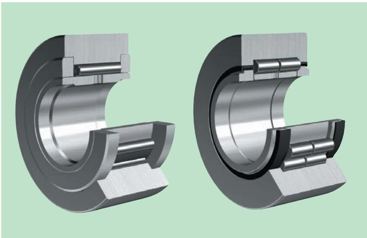
This roller follower is a bearing designed for rotation of the outer ring. A needle roller and cage assembly, an inner ring, and a face ring are assembled in a thick-walled outer ring.
