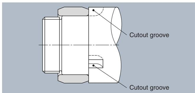
**Fig. 8.4** Cutout groove for inner ring extraction
