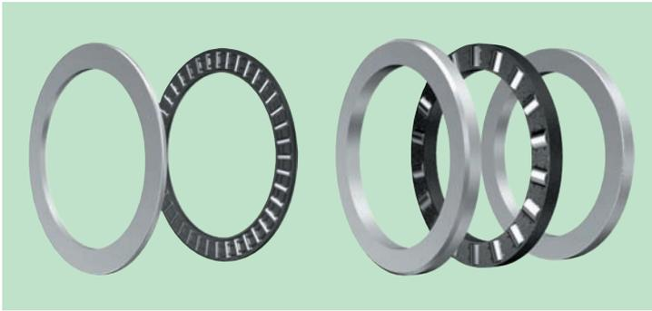
The product is comprised of needle or cylindrical rollers, a cage that guides and retains the rollers, and a disk shaped bearing ring, and is capable of holding an axial load in one direction. The mounting surface can be used as raceway surface when the mounting surface are beat-treated and finished. As a result, the bearing can be supplied without bearing ring raceways.
