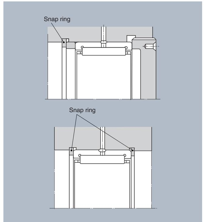
**Fig. 8.10** Outer ring fixing method with snap ring
