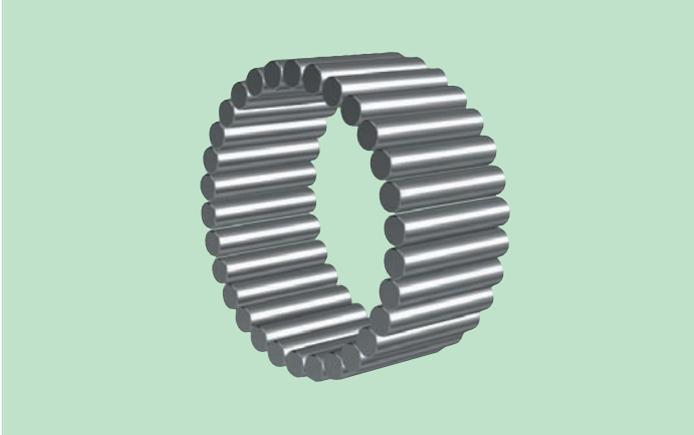
The needle rollers with flat end round end faces are standard. These rollers are made of high-carbon chrome bearing steel, surface-finished by grinding and buffing after heat-treatment.
