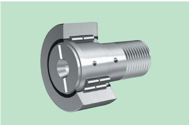
This is a full complement roller bearing designed for rotation of the outer ring. Double-row cylindrical rollers and a stud instead of inner ring are fitted in the thick-walled outer ring. The stud is threaded to be mounted easily.
